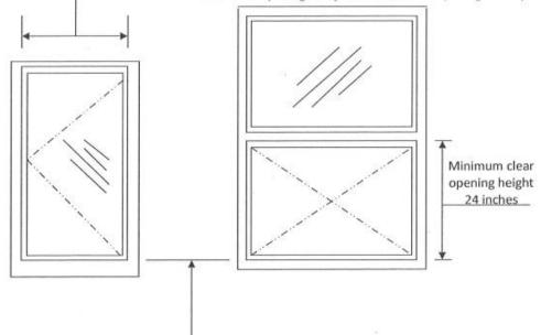
Emergency escape and rescue opening cannot be located more than 44 inches above the floor. The measurement is to be taken from the floor to the bottom of the clear opening.
