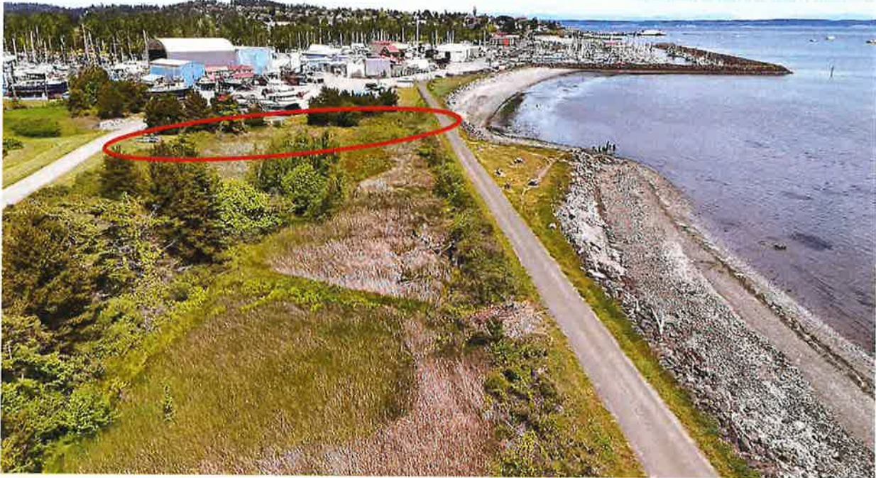
Photo 4. Study area facing north. The flow spreader embankment (circled in red) stretches from 8th Street to the Larry Scott Memorial Trail, separates Wetland A from the Boatyard. The Study Area is confined by 8th Street (left) and the Larry Scott Trail (right).
