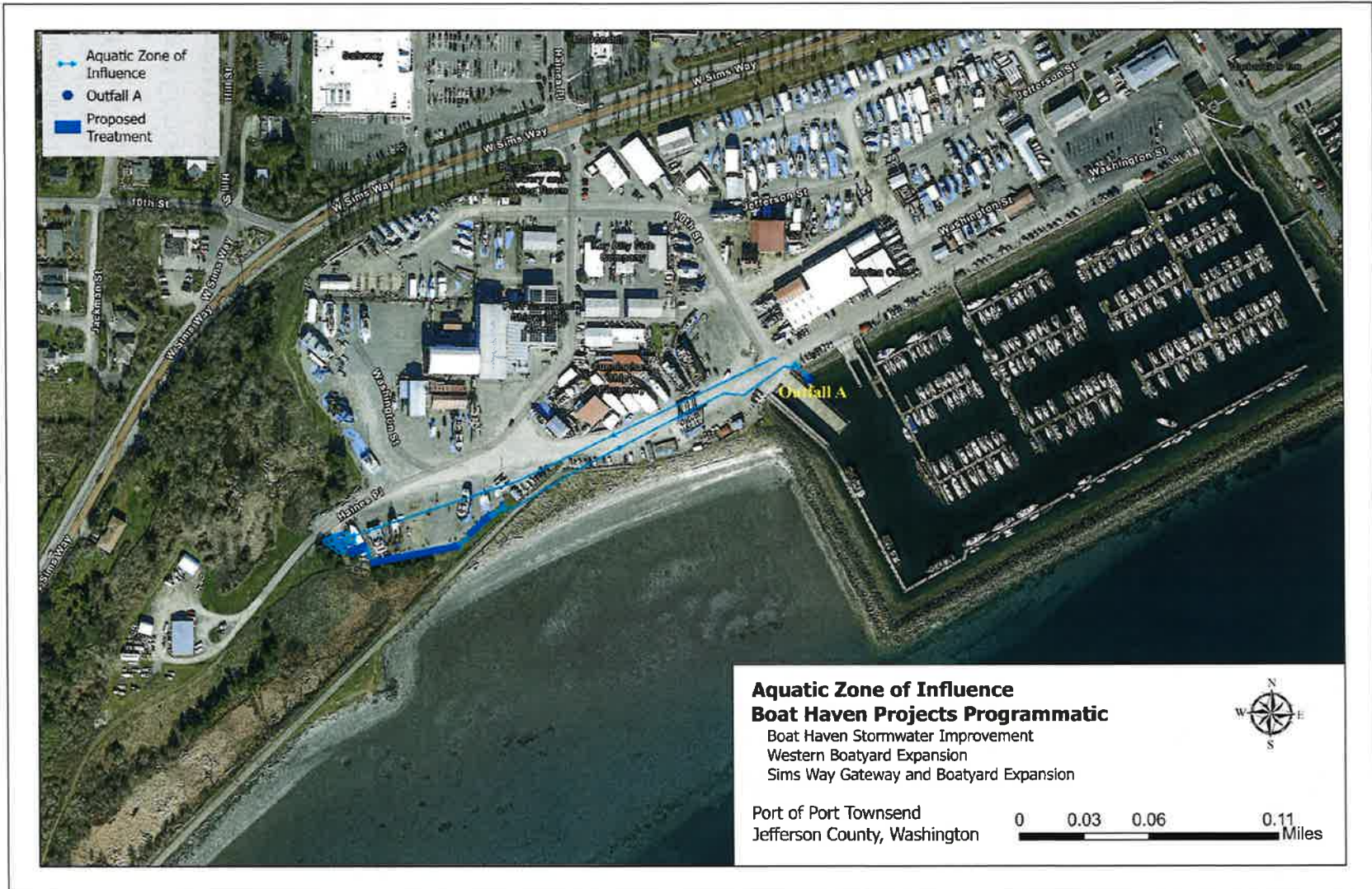
Figure 4. The Aquatic Zone of Influence, defined by the extent of stormwater effects, will be restricted to the installation of the new 4-stage biofiltration treatment system which will reduce the baseline discharge of pollutants to Port Townsend Bay from the Boat Haven Boatyard through Outfall A.
