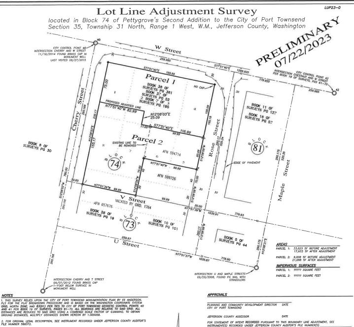
3. THIS SURVEY COMPLIES WITH W.A.C. 332-130-100 AND WAS ACCOMPLISHED IN JULY, 2020 BY FIELD TRAVERSE METHODS USING A TOPCON GPT 9001A 1-SECOND ROBORIC TOTAL STANON CALIBRATED AT THE CALLAM COUNTY BASELING ON MARCH 20, 2023, SOME DISTANCES MEASURED WITH A STEEL TAPE.
